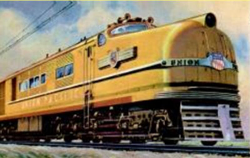
Progress of American railroads is demonstrated in these photographs of the latest locomotives. Left, giant steam-electric power car which the Union Pacific had built for service on long runs
