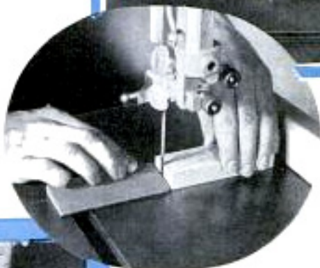
A strip nailed to a board with irregular edges enables it to be guided properly past a circular saw
