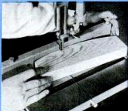
Strips are cut to a uniform arc by using the ripping fence, which is marked at the pivoting point
