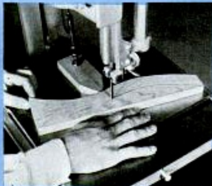
If a curved part is of uniform width, the second cut is made by clamping a pivot opposite the blade
