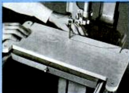
Cutting a sidepiece for the jig. In this type of ripping, the fingers of one hand serve as a pivot
