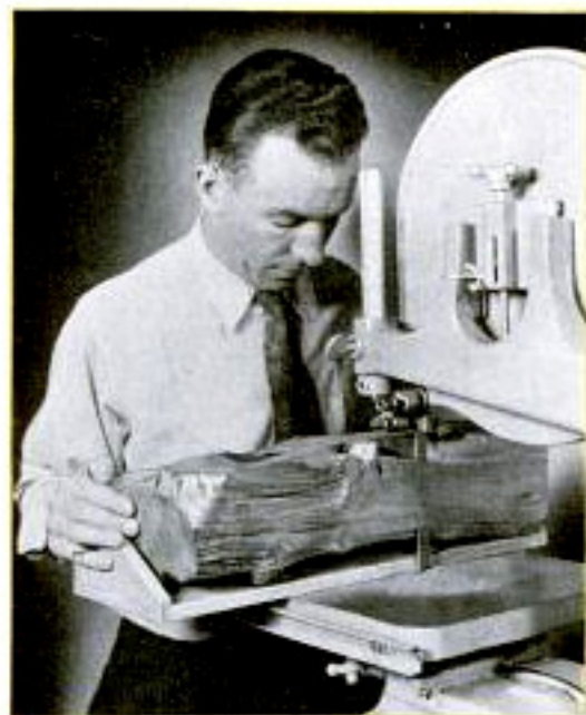
For trimming two opposite sides, rough pieces are held in a cradle
