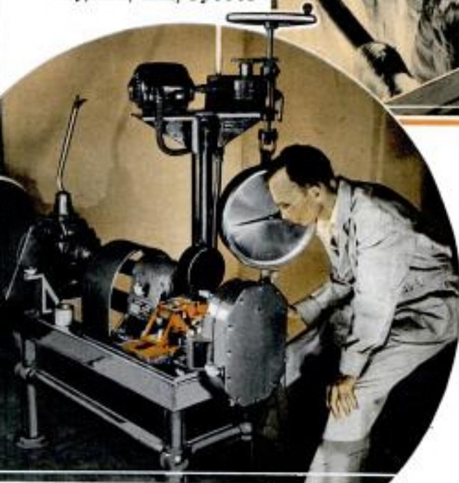
RUNNING test an extreme-pressure lubricants, developed through the wizardry of the chemist. Above, inspecting rayon, a man-made fabric produced by chemistry.
