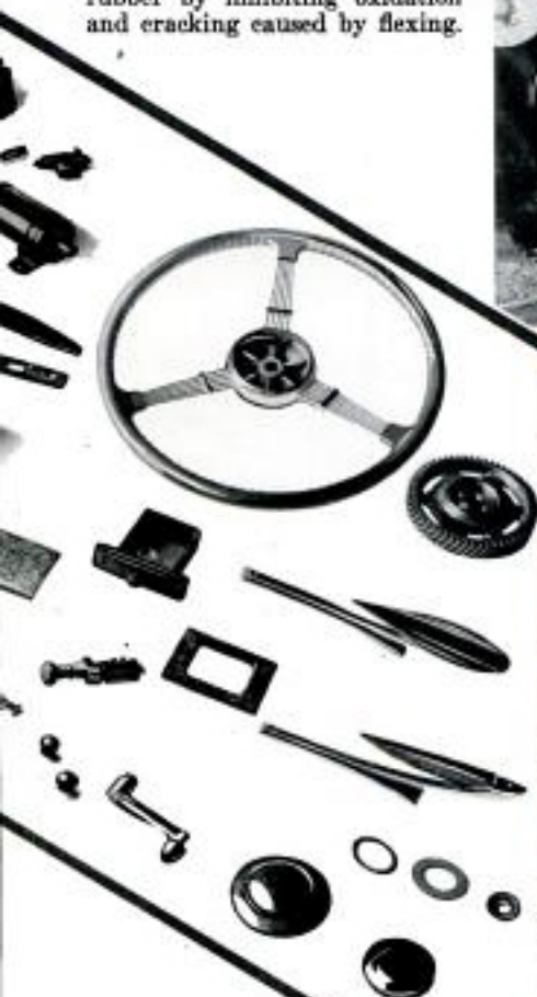
PLASTIC materials used in Hudson car, including wheel, ignition parts, timing gear and washers, interior fittings and radiator ornament.
