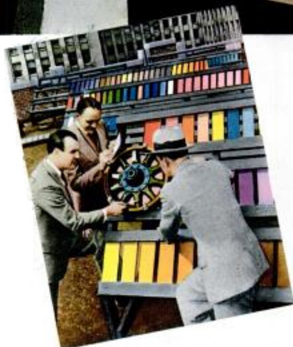
RACKS on roof for making exposure tests of finishes. Above, examining paint and lacquer samples for cracks or other imperfections.
