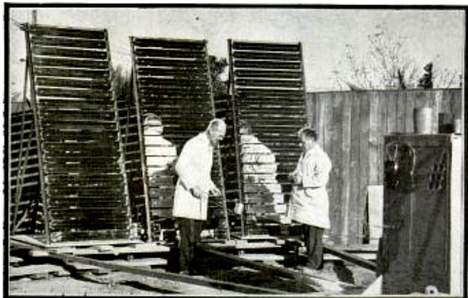
Sets of Mirrors with Which the Sun's Rays Are Focused to Produce Extremely High Temperatures; Heat as Great as 50,000 Degrees May Be Obtained in This Manner, the Inventor Claims
