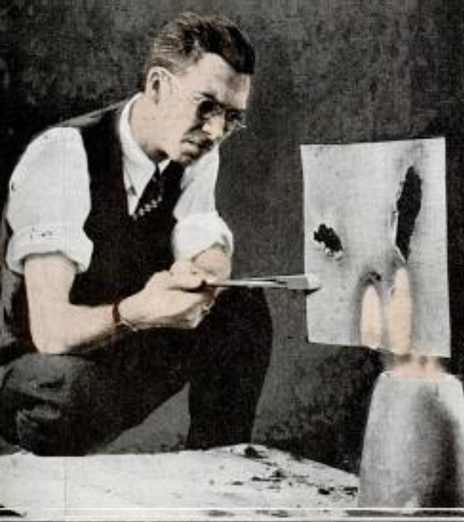
Left, melting a metal sheet with the aid of concentrated heat from a solar furnace
