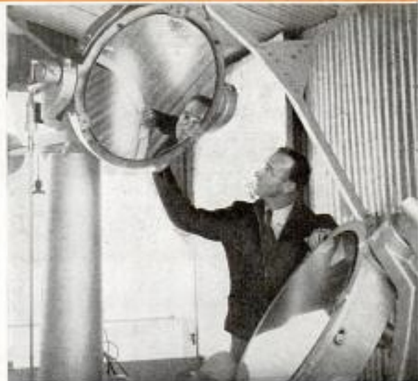
Top, studying sunspots on paper disk suspended in light path of solar telescope, and examining sunspots on glass negatives made with aid of telescope. Below, mirror dishes of horizontal telescope used to study sun
