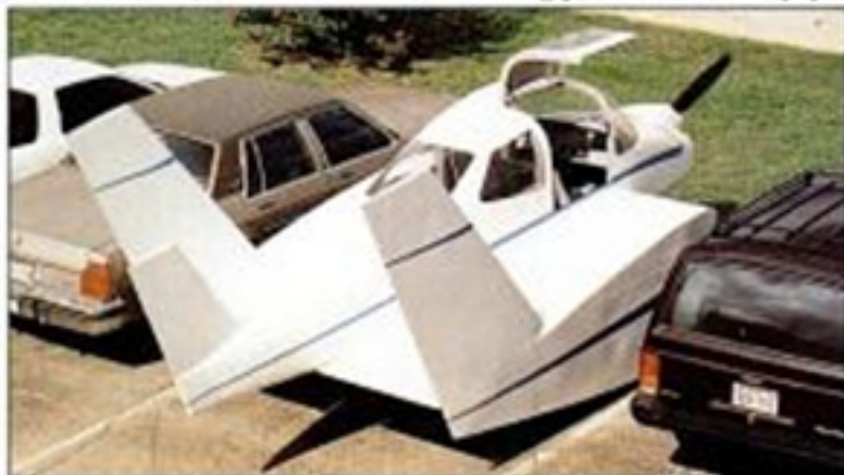
At motorhome width, proof-of-concept mockup fits within confines of a parking space.
