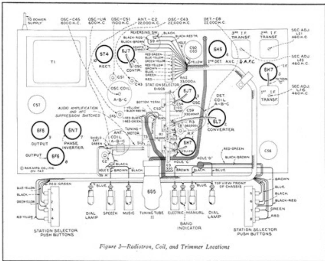
Figure 3—Radiotron, Coil, and Trimmer Locations
